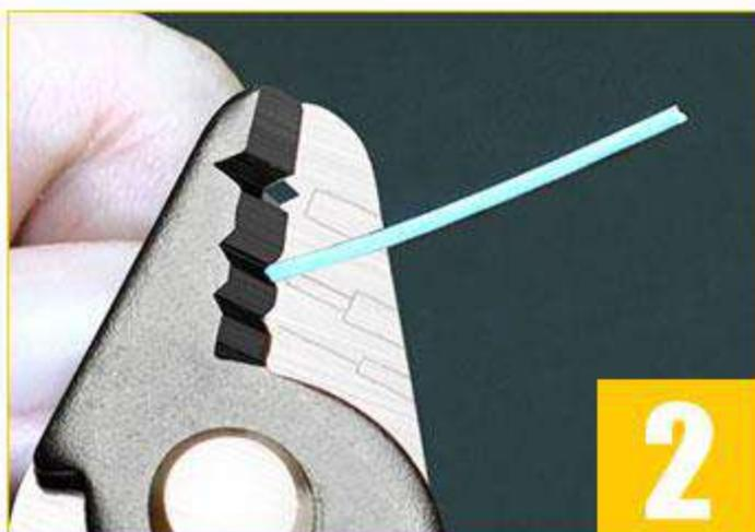
Strips the **600~900 $\mu\text{m}$**  buffer coating down to the **250 $\mu\text{m}$**  coating.
