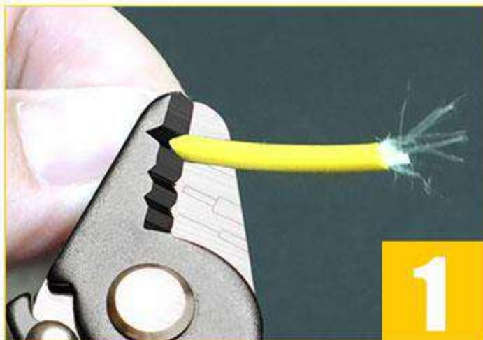
Strips the **1.6-3.0mm** fiber jacket down to the **600-900  $\mu\text{m}$**  buffer coating
